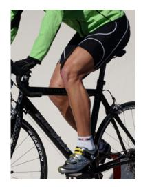
The neutral knee position serves as a good starting point for most cyclists, though many adjust it from here: long distance (stage) racers and mountain bikers often move the saddle back by 1cm or more, for power, and sprinters may move it forward, "getting on top of the gear" for quick acceleration.
